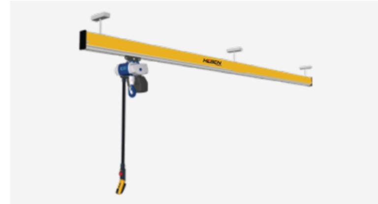
Straight Monorail provides a straightforward and efficient solution for moving materials along a dedicated path. They consist of a single beam (I-beam, box section, or profile type) supported by pillars, along which a hoist travels. Straight monorails are ideal for point-to-point transport of loads up to 12.5 tons over distances up to 12 meters. They offer a simple, adaptable solution with manual or powered travel options.
